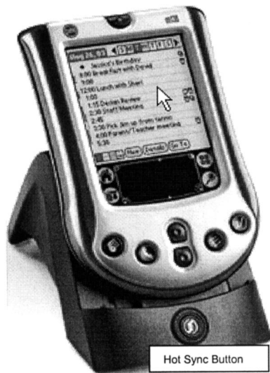
Fig. 4. Palm M-130 personal digital assistant in its cradle, ready to download data. The cradle also recharges the Palm M-130's batteries.
