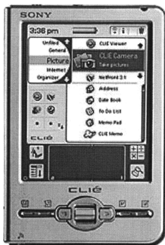
Fig. 1. One type of handheld computer (also known as a personal digital assistant or PDA) useful for storing, manipulating, and accessing various types of medical information.
