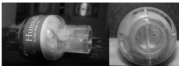
Fig. 2. Heat and moisture exchanger nearly completely occluded by mucoid secretions.
