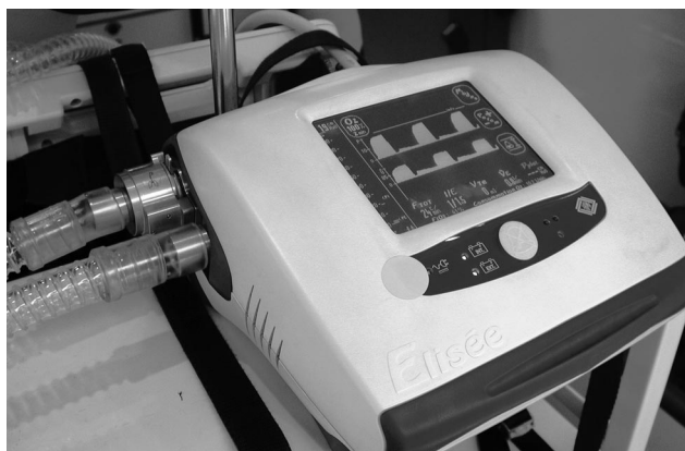
Fig. 2. The Elisée 250 transport ventilator. The ventilator settings are adjusted chiefly via the touch-pad, which has 4 display screens, each dedicated to one function: mode selection, machine parameter settings, alarm settings, patient monitoring (screen shown in this picture). The on/off button is on the side of the ventilator and is not visible in this picture. A lit button under the screen signals alarms visually and allows for the turning off of alarm sounds.
